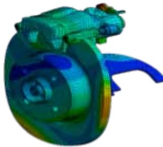
Analysis of brake assembly for brake squeal: Combining nonlinear pre-stressing of structures and complex unsymmetric eigensolvers leads to accurate analysis.
