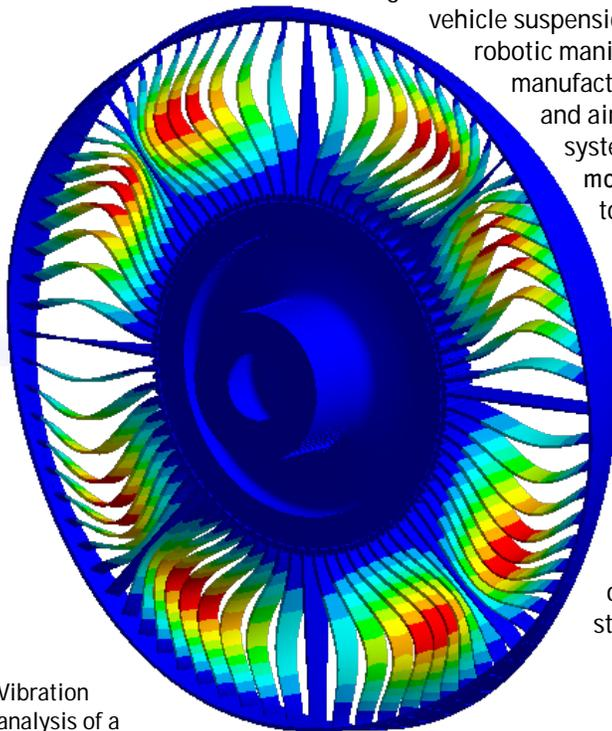
Vibration analysis of a bladed disc using cyclic symmetry
