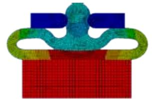
Large deformations and contact analysis of a rubber seal. ANSYS material models include elasticity as well as visco-elasticity, plasticity, viscoplasticity, cast-iron plasticity, creep, hyperelasticity, gaskets and anisotropy.
