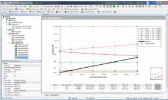
Campbell diagrams identify critical speed of rotating structures over a range of variations of a system's rotational velocity.
