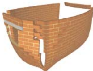
Damage and collapse of a brick building due to an internal explosion
