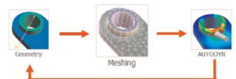
Typical Workflow with parametrically linked ANSYS AUTODYN in ANSYS Workbench
