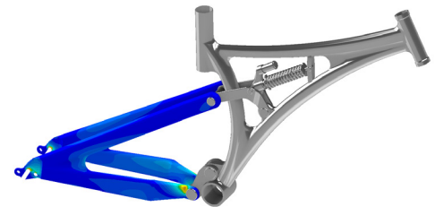
Equivalent stress results in a mountain bike frame assembly
